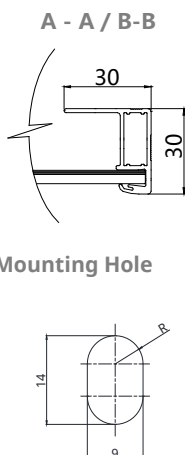
Frame Cross Section
